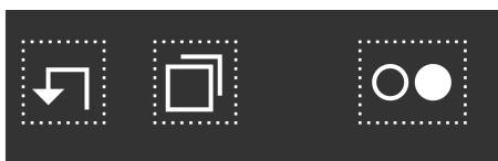
Figure 7: Sensor buttons on the device for navigating the display pages of the main menu level and master button
