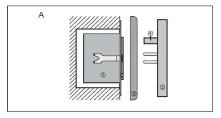
The connecting terminals of the insert must be down. Do not use the relay insert when not in combination with a cover. Plug cover (2)onto the insert together with frame (3). Electrical contacting is established through plug (4). Plug on the cover prior to switching on the mains voltage. Mains failures of more than 1 sec. will lead to switching off the relay insert.
