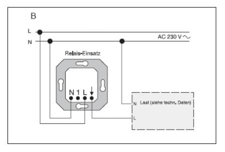
Connect the relay insert as shown in Fig. B. Relay insert (5), Load (6) Observe the maximum connected load and the specified load as per Specifications. Depending upon the type of installation, reduce the maximum connected load by:
